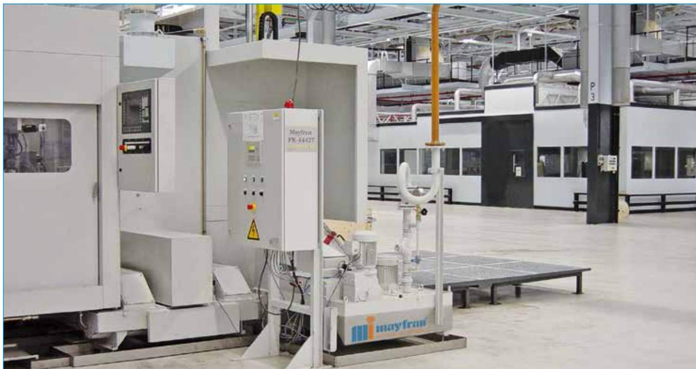
Machine pump station directly on the machine with supply to the Viavent overhead system
