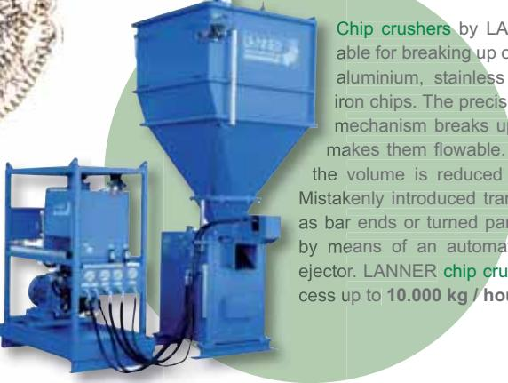
**Chip crushers** by LANNER are suitable for breaking up oily, woolly steel, aluminium, stainless steel and cast iron chips. The precision grinding tool mechanism breaks up the chips and makes them flowable. In the process, the volume is reduced by up to 80%. Mistakenly introduced tramp metals such as bar ends or turned parts are removed by means of an automatic tramp metal ejector. LANNER **chip crushers** can process up to **10.000 kg / hour**.
