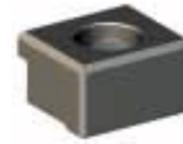
CHICK Toe Clamps (four per set) provide the quickest and most secure means of mounting a Qwik-Lok to a T-Slotted VMC table. Toe clamps are designed to be used with either 1/2-13 or M12 socket head cap screws.
